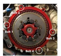
FIG 4. Dry clutch without OE cover
