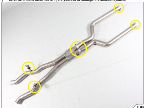
! IMPORTANT: mark the front link pipes, 45 mm (1,77 in) from the beginning, for later adjustments (F 04, 05).
