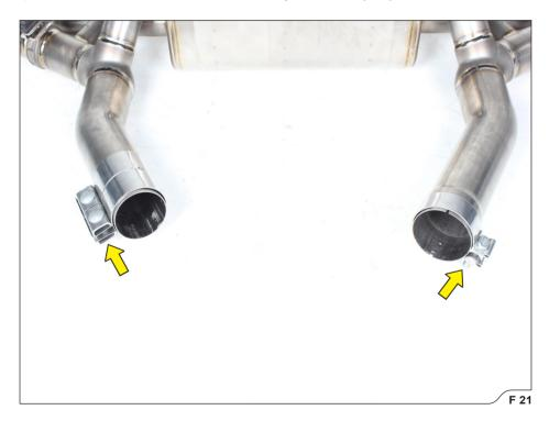
! IMPORTANT: unscrew the double clamp's nuts enough, to be able to slide the clamp completely onto the pipe (F 22)!
