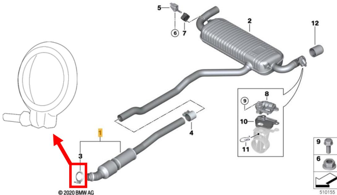
On older models there was a different connection between stock downpipe and link-pipe. Instead of the »V-clamp« mentioned above the »overlapping« connection was used- see schematic below. On this vehicles unfortunately Akrapovic link -pipe E-BM/SS/6 will not fit because of different joint.
