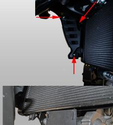
2. Remove the rubber protection rubber as shown in the picture
