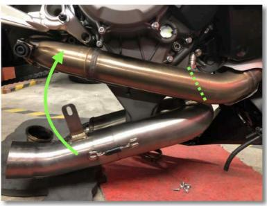
• Fit the De-cat the same way the Cat-box was removed. Firstly bolt up the front brackets just finger tight, using the supplied 2x M8 x 25mm Hex head bolts along with the 2x rubber mounts with washers. The rubber mounts fit within the front brackets.
