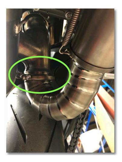
Using the stock clamp, clamp up the inlet flange of the De-Cat to the outlet flange of the stock header, making sure the parts have correct alignment and that no part of the clamp can come into contact with the under side of the swing arm.
