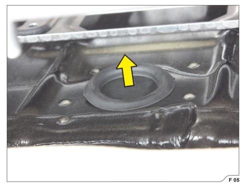
Open the trunk and remove the marked trunk trim and floor panel to get access to electrical wiring harness in the trunk; check vehicle manufacturer manual for correct trunk panels/floor disassembly (F 06, 07, 08, 09, 10, 11).
